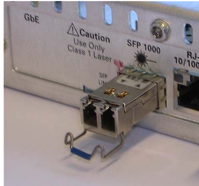
Figure B-8: SFP module - Dismounting
